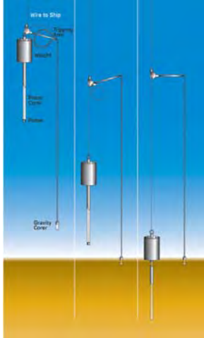
Figure 8 Piston Corer Source: Woods Hole Oceanographic Institution
