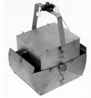
Figure 4: Ekman Sampler Source: NJDEP Field Sampling Procedures Manual (2005)
