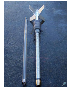
Figure 6 Gravity Corer Source: Mooring Systems, Inc.
