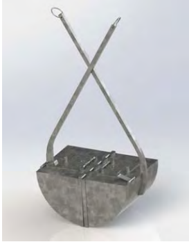
Figure 3 Van Veen Sampler Source: GrabCAD.
